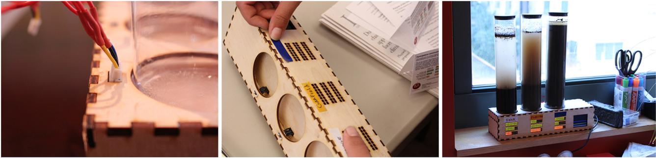
**Figure 2. Designing a bio-electronic system: column plugged into casing; labeling the column slots; testing the system.**
