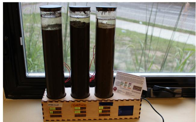
Figure 1. Bio-electronic soil sensing device deployed at an environmental outreach community center.
